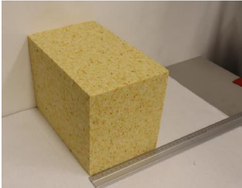
Sample for emissions testing of bonded postconsumer mattress foam
