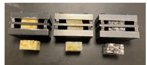
Compression set testing
