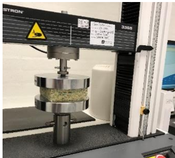
Compression load deflection testing
