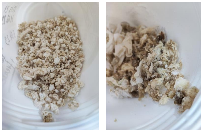
Figure 2 Diapers disintegrated in Laboratory before fermentation test (compostable – left, conventional – right).
